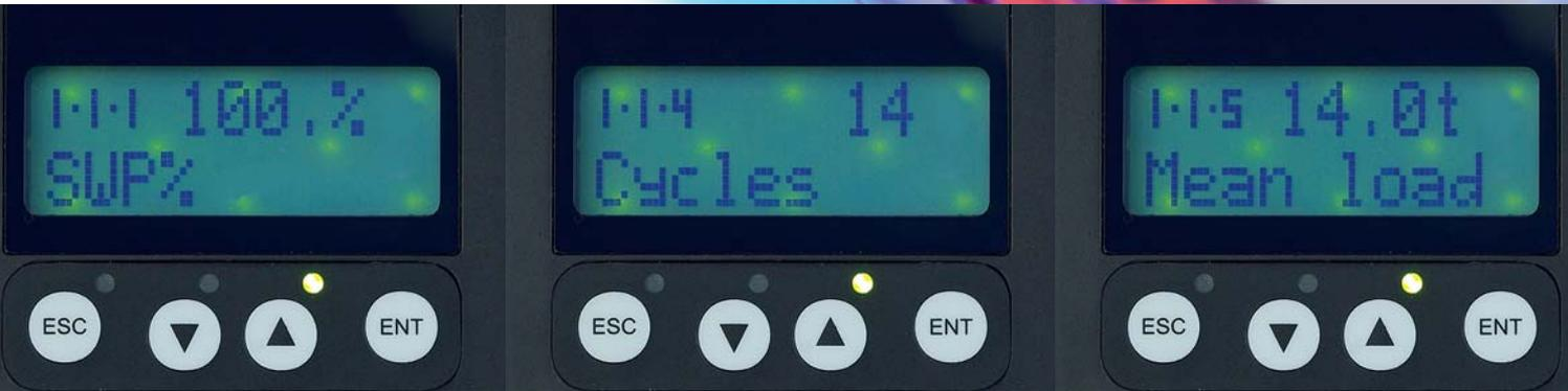
The optional display unit can be mounted on the control pendant and the load display (accuracy  $\pm 5\%$ ) caters for an optional tare weight function. The programming of the crane as well as the reading of the actual operation values can all be done via the push button pendant. This enables the operator to quickly and easily check the crane's status.
